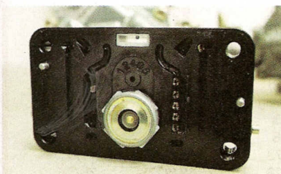
The Ultra-series Holley carbs feature billet baseplates and metering blocks, and have these adjustable emulsion bleeds that can help tune street driveability to perfection.
